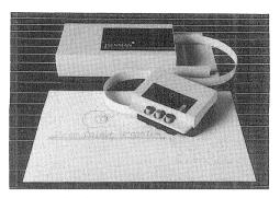
the plotter and the wheels beneath. A flat ribbon cable about a metre long also unreels - this is the Penman's umbilical cord. The package design is of the highest order.
